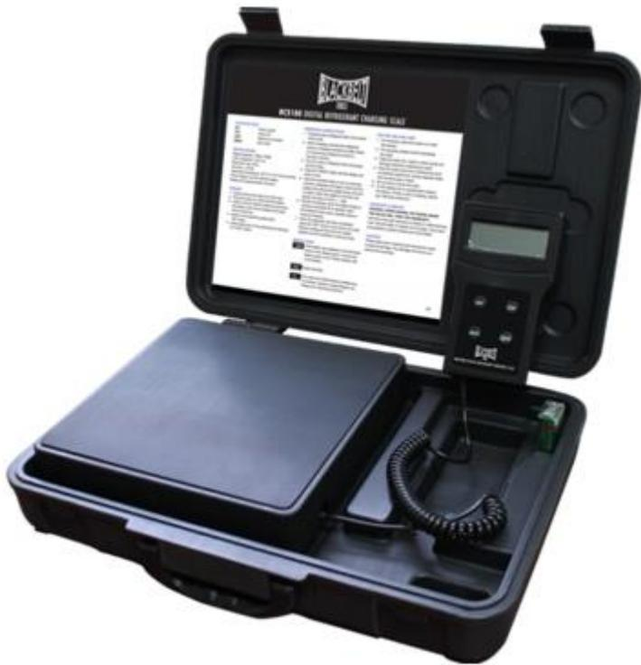
Carrier ductless systems requires all refrigerant to be weighed into the system prior to the service valves being opened. The amount of refrigerant will vary from system to system. The additional charge needed can be found in the specific products installation manual and is based on oz. per lineal ft. over a predetermined length that the factory charge will handle.
