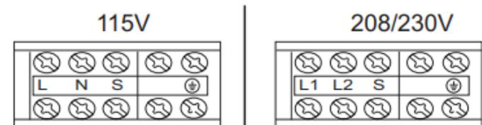
**Fig. 14 — Control and Power Wiring on Indoor Unit**
