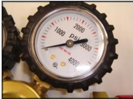
Carrier Enterprise requires a 500 psi dry nitrogen pressure test on ***all*** DLS system refrigerant piping. *You may find some manuals stating a 150 psi pressure test, this is a cooling only system guideline and should technically still have a 500 psi pressure test.*
