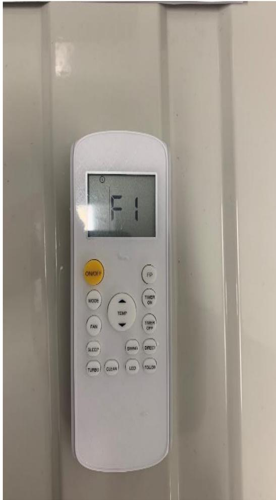
Reinstall the batteries within 30 seconds of replacing batteries, simultaneously press mode and timer on for 5 seconds. This is service function mode and should read F1
