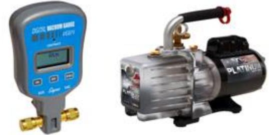
7. When micron gauge reaches 1000, close vacuum pump valve for rise test. Micron level should rise a bit but **MUST** eventually stop rising for 15 minutes.
